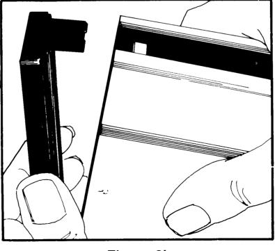
**Figure 3b** Carefully remove the end cap from the Smartmodem.
