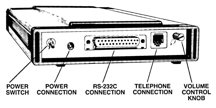
Figure 2 Smartmodem Back Panel
